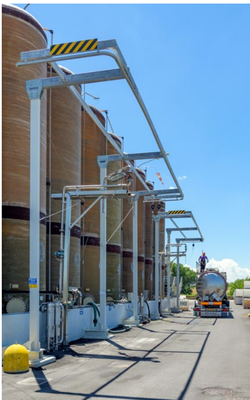
Truck Solution with custom cantilevered modular extension.
